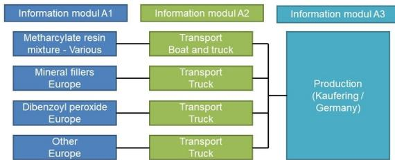
**Illustration: Production process of the reaction resin mixture**
