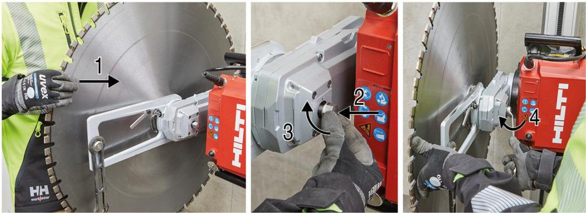
1. Turn the blade guard holder in the direction from which you want to insert the saw blade with inner flange.
