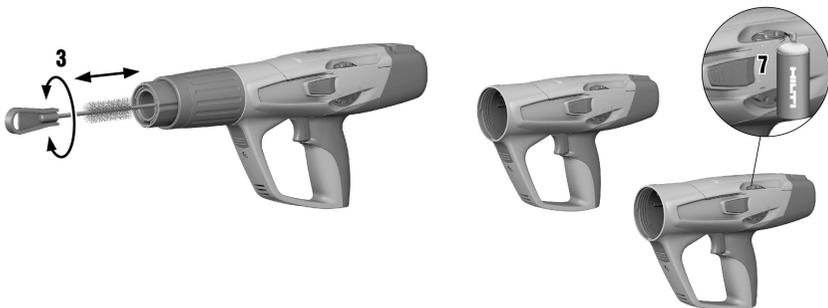
1. Spray the piston rings lightly with oil and then use the flat brush to clean them using the flat brush until the rings are free to move.
