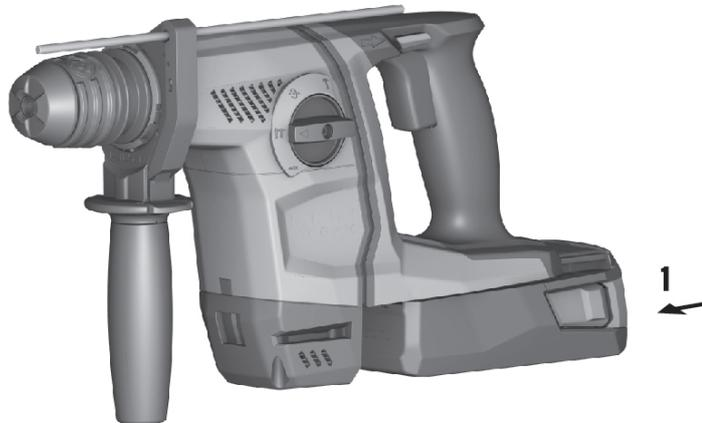
1. Push the battery into the battery holder until it engages with an audible click.
