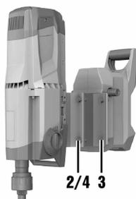
1. Detach the diamond core drilling machine from the drill stand.
