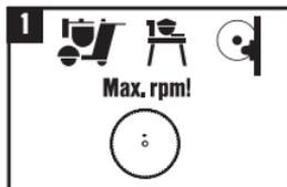
The speed (RPM) listed on the accessory must be higher than the speed of the tool. If in doubt, the maximum peripheral speed of an accessory is 80 m/s.
