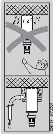
Use of the water collection system in conjunction with a wet-type industrial vacuum cleaner is a mandatory requirement for working on ceilings.
