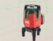
激光标线仪及激光投点仪
